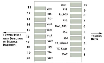
Figure 2: Interface to Host PCB
