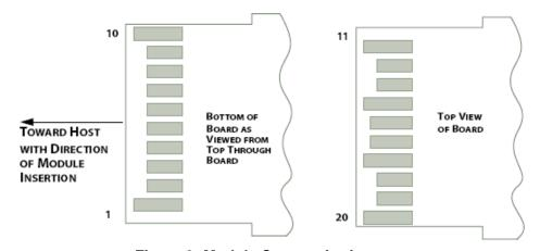
**Figure 3: Module Contact Assignment**
