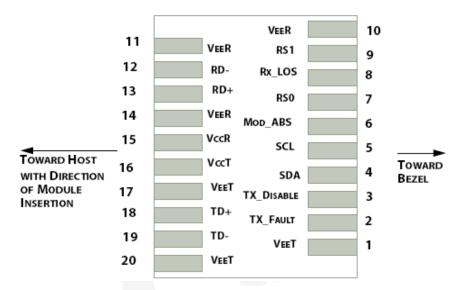
Figure 2: Interface to Host PCB
