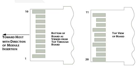
Figure 3: Module Contact Assignment
