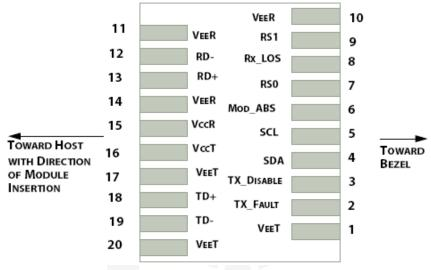
Figure 2: Interface to Host PCB
