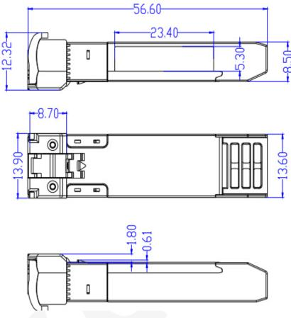
**Figure 4. Mechanical Specifications**
