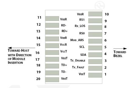
Figure 1. Electrical Pin-out Details
