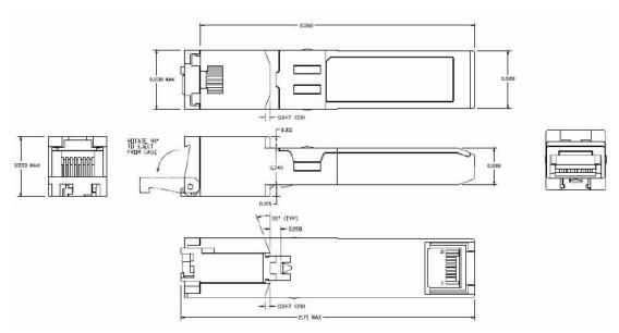
Figure 2. 6C-SFP-M mechanical dimensions
