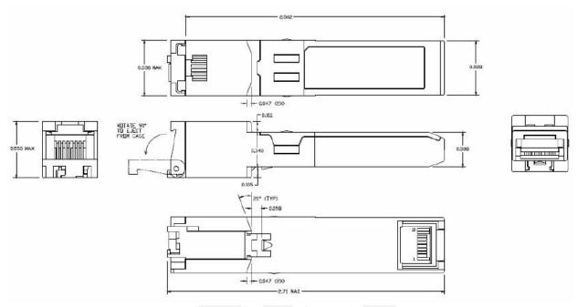
Figure 2. 6C-SFP-F mechanical dimensions
