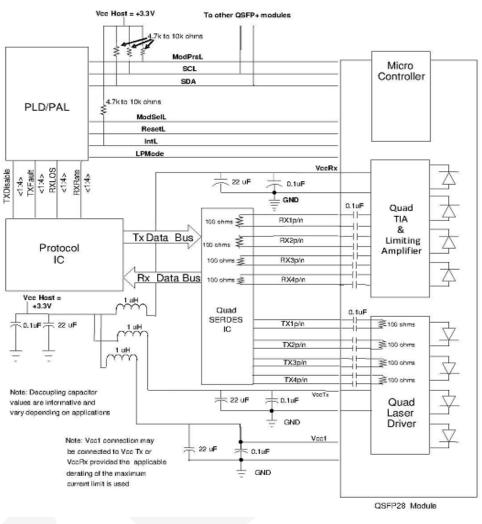
Figure 4. Host - Transceiver Interface Block Diagram
