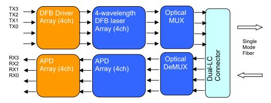
Figure 1: 40Gb/s QSFP ZR4 Transceiver Block Diagram
