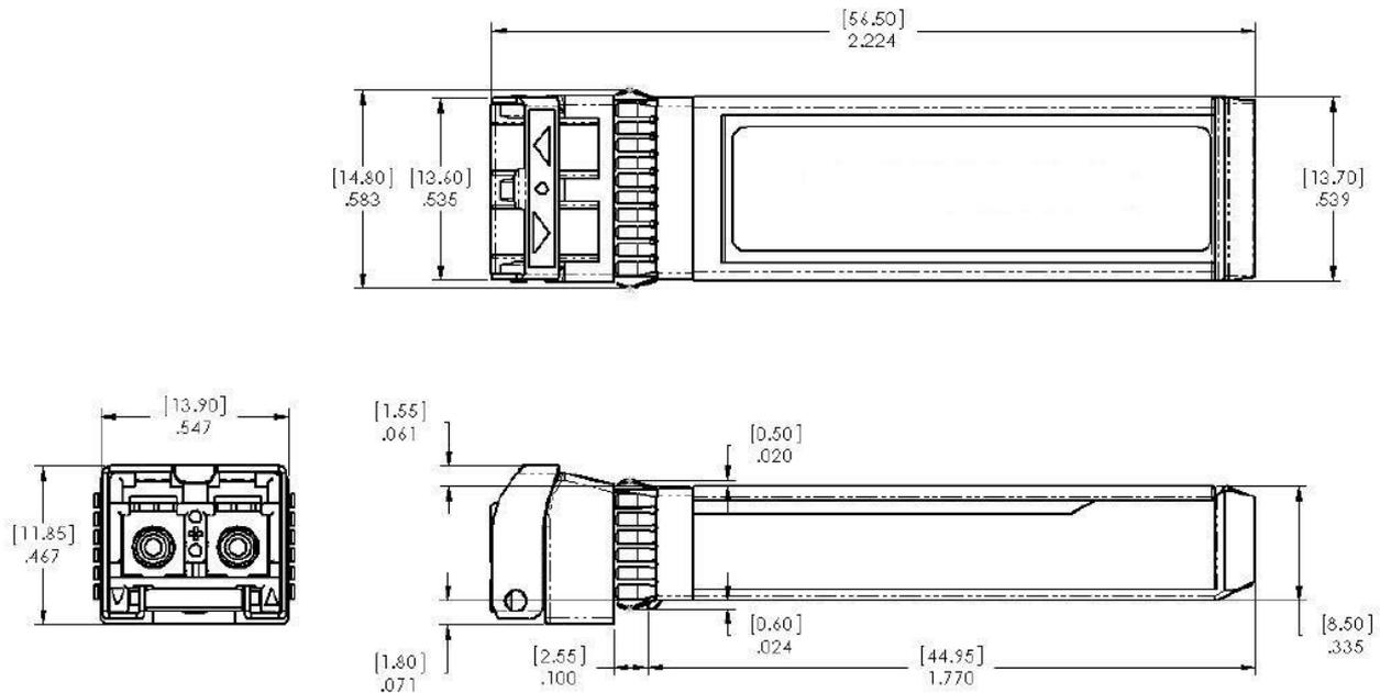
Figure 3. Module Mechanical Dimensions
