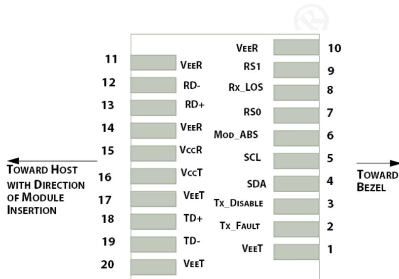
Figure1.Electrical Pin-out Details
