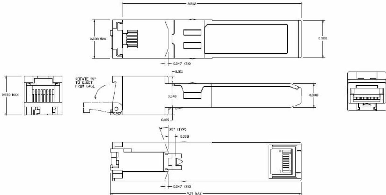
Figure 2. 6C-SFP-T mechanical dimensions
