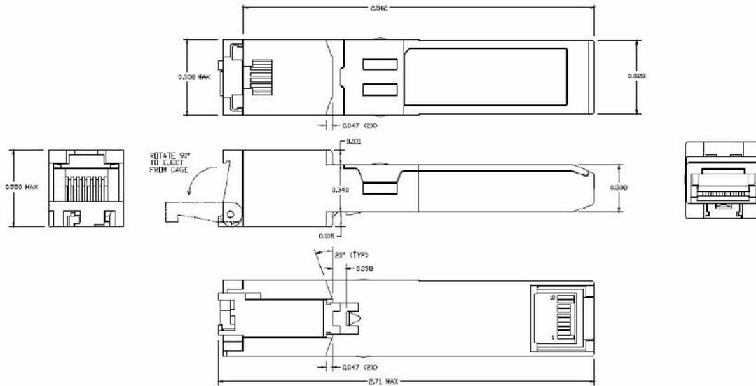
Figure 2. 6C-SFP-M mechanical dimensions
