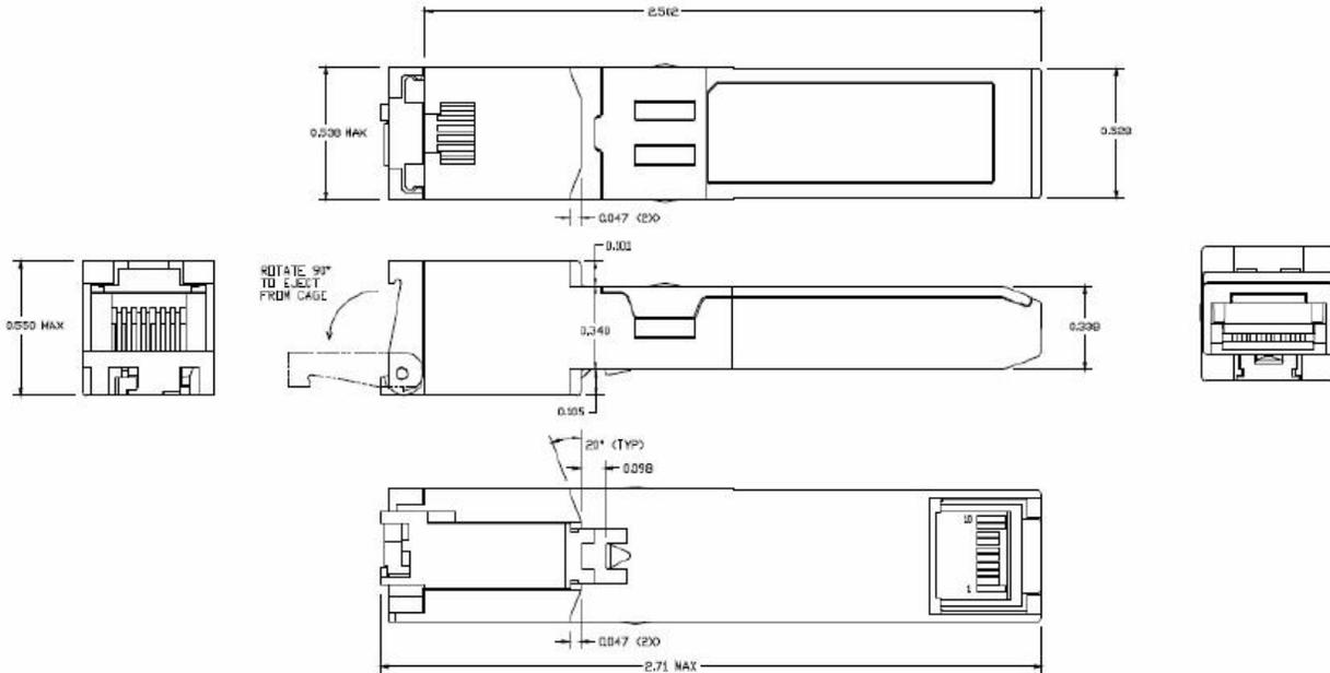
Figure 2. 6C-SFP-F mechanical dimensions
