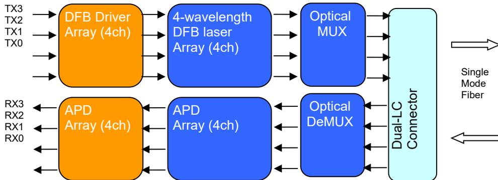
**Figure 1: 40Gb/s QSFP ZR4 Transceiver Block Diagram**
